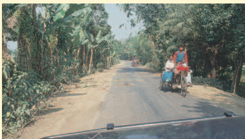
The final product, a Single Otta Seal after 2 years in service. (Bangladesh).
