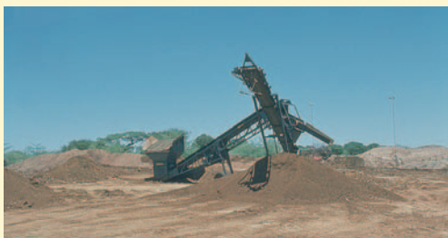
“As dug material” which in many cases only requires screening of oversize materials, can successfully be used in Otta Seals. (Kenya).
